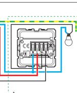
Attention, the dimmer must be installed on the lamp side
