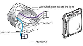
Use a connector to connect all 3 wires together (travellers 1 and 2 and lamp return wire). Use an other connector for neutral wire.
