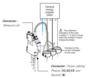
A circuit breaker from C2 to C16 rating is required according to the cable cross section used to supply the three-phases energy meter. The connection between the three-phases energy meter and the coil is made via a connector.
