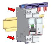
2. Pull the device forward in order to release it from the DIN rail
