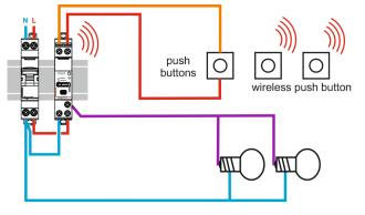
. Wireless installation with several wireless push-buttons " ... with
