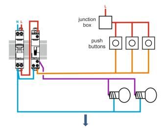
After: Installation « 3 wires » with line on the push-buttons
