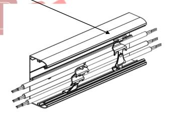
The clip allows the reserve of the cables under installation
