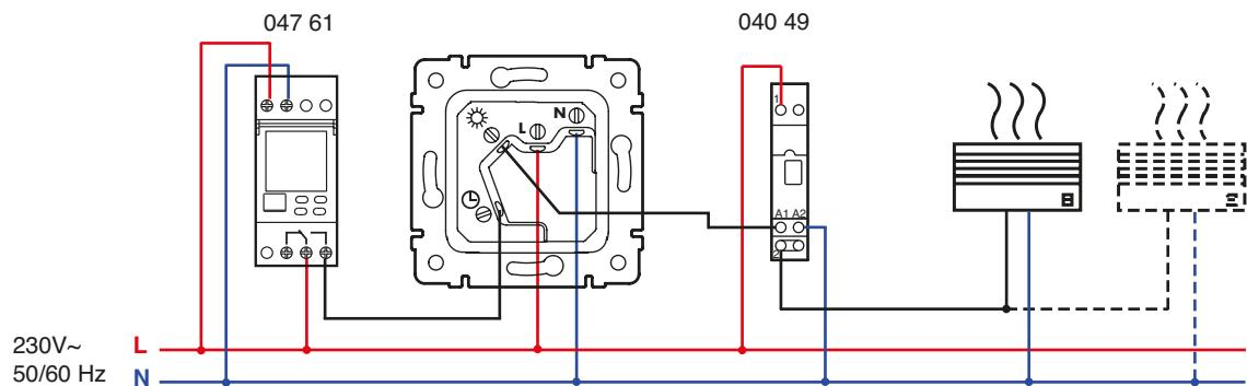
• **Attention:** Distribution voltage to be connected cophasally to thermo regulator and remote control. Installation and assembly may only be effected by an expert!
